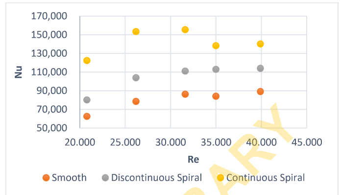
Figure 6: Average Nusselt numbers of the test channels
