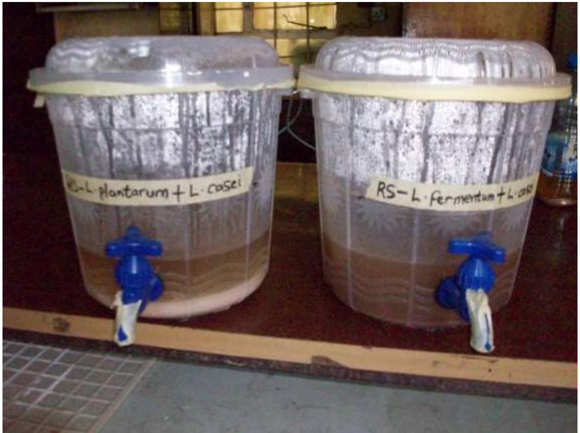
Plate 4.2: Improved fermentors for the fermentation of the wort from the different sorghum varieties.
