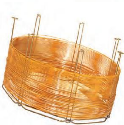
Plate 2.6. Gas chromatography capillary columns (Source; Agilent J & W GC columns)
