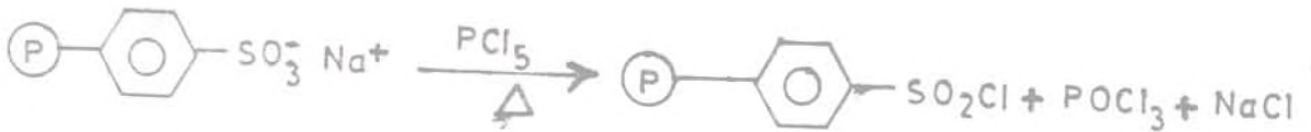
Fig. 1.39: Equation illustrating conversion of sulphonated ion exchange resin (sodium form) to the sulphonyl chloride form
