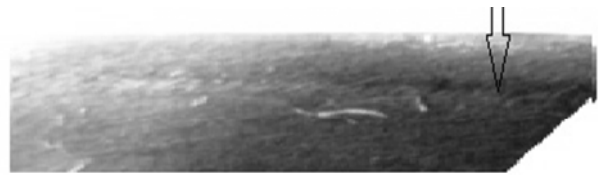
Figure 2. Segmented top portion of macro-etched lead sample with arrow showing shear line running across plate caused by upper roll after two passes.
