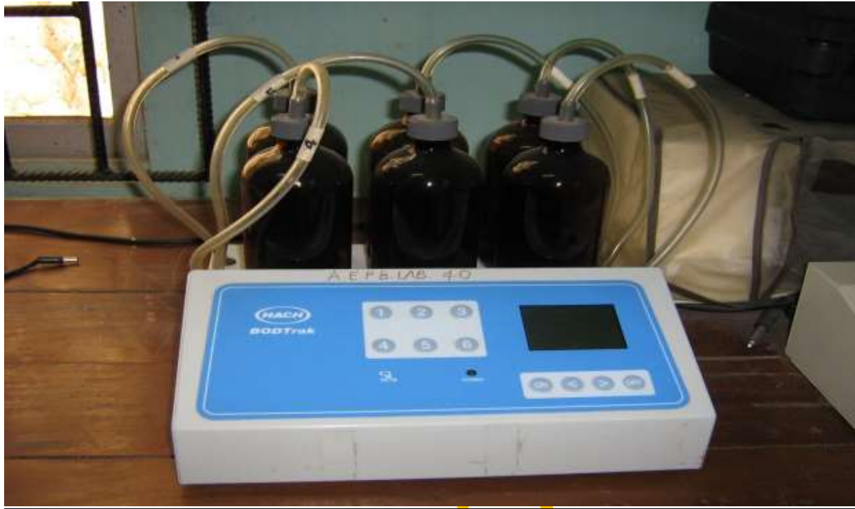
Plate 15: BOD equipment used for the analysis
