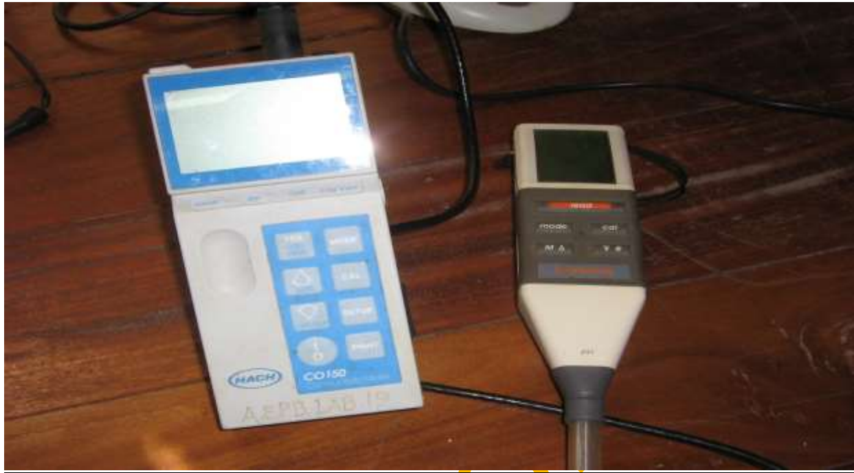
Plate 19: Oxygen meter used in the determination of dissolved oxygen
