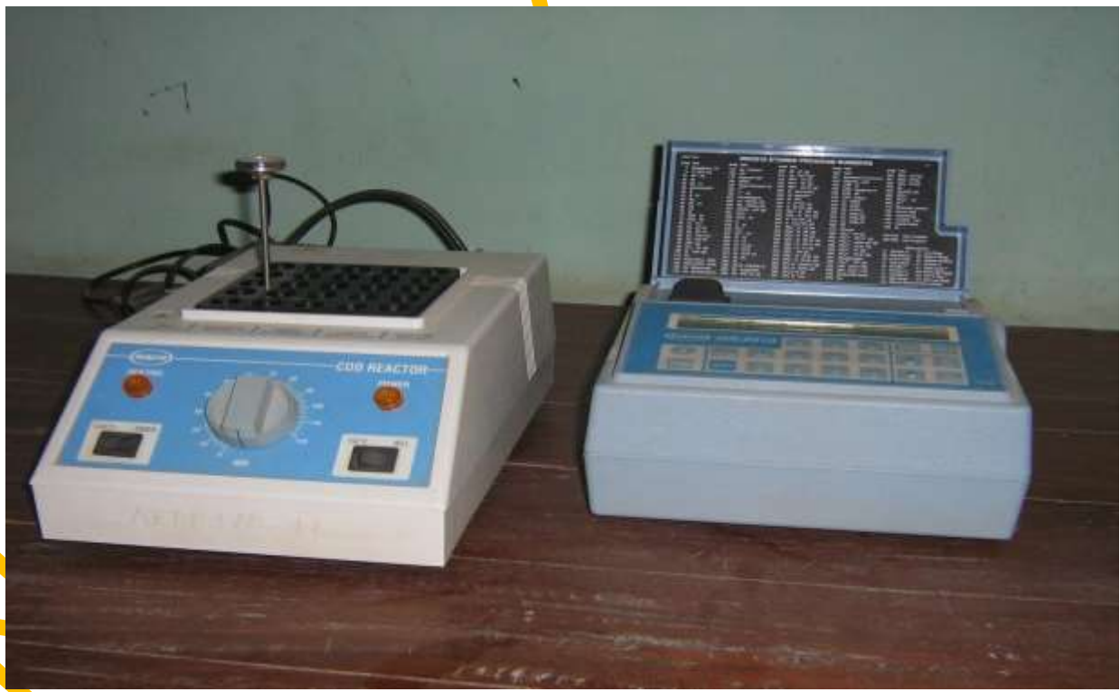
Plate 16: COD equipment for analysing samples in this study
