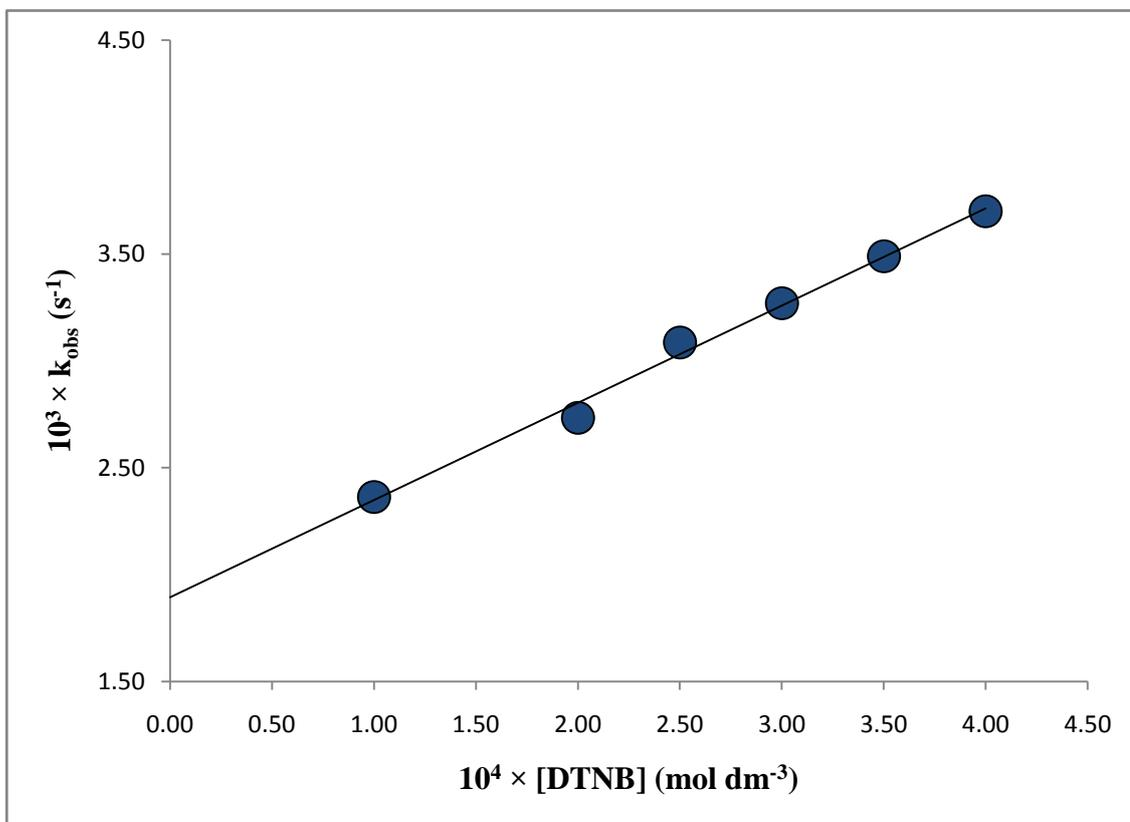
**Figure 4.27:** The dependence of the pseudo-first order rate constant,  $k_{\text{obs}}$ , on the DTNB concentration for the reaction of DTNB with *stripped human deoxyhaemoglobin A* at 25°C.
