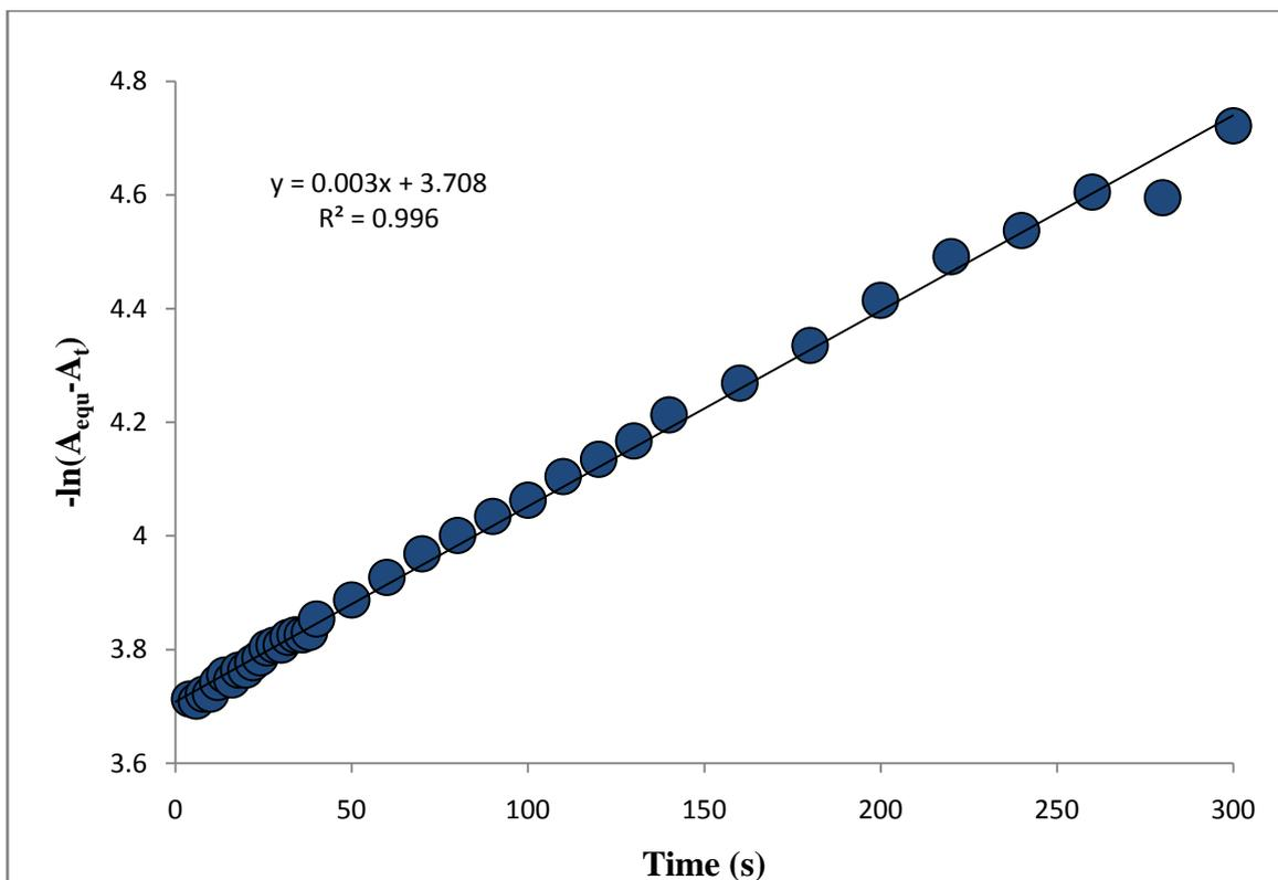
**Figure 4.25:** Semi-logarithmic plot of the time course for the reaction 5,5'-dithiobis(2-nitrobenzoate) with *stripped human deoxyhaemoglobin A* sulphhydryl groups in borate buffer pH 8.00;  $[DTNB] = 250 \mu\text{mol dm}^{-3}$ ;  $k_{\text{obs}} = (3.45 \pm 0.04) \times 10^{-3} \text{ s}^{-1}$ . The plot was linear for 1.5 half lives. Data from Figure 4.22.
