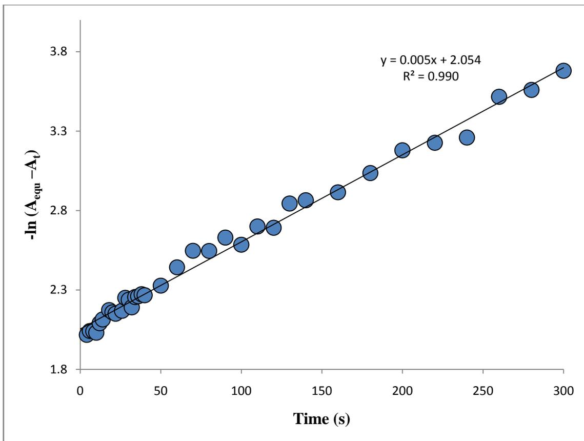
**Figure 4.34:** Semi-logarithmic plot of the time course for the reaction 5,5'-dithiobis(2-nitrobenzoate) with the *minor cat oxyhaemoglobin* sulphhydryl groups **in the presence of inositol- $P_6$** ; phosphate buffer **pH 6.04**;  $[DTNB] = 400 \mu\text{mol dm}^{-3}$ ;  $[\text{inositol-}P_6] = 10 \mu\text{mol dm}^{-3}$ ;  $k_{\text{obs}} = 5.48 (\pm 0.09) \times 10^{-3} \text{ s}^{-1}$ . The plot was linear for 2.4 half lives. Data from Figure 4.29.
