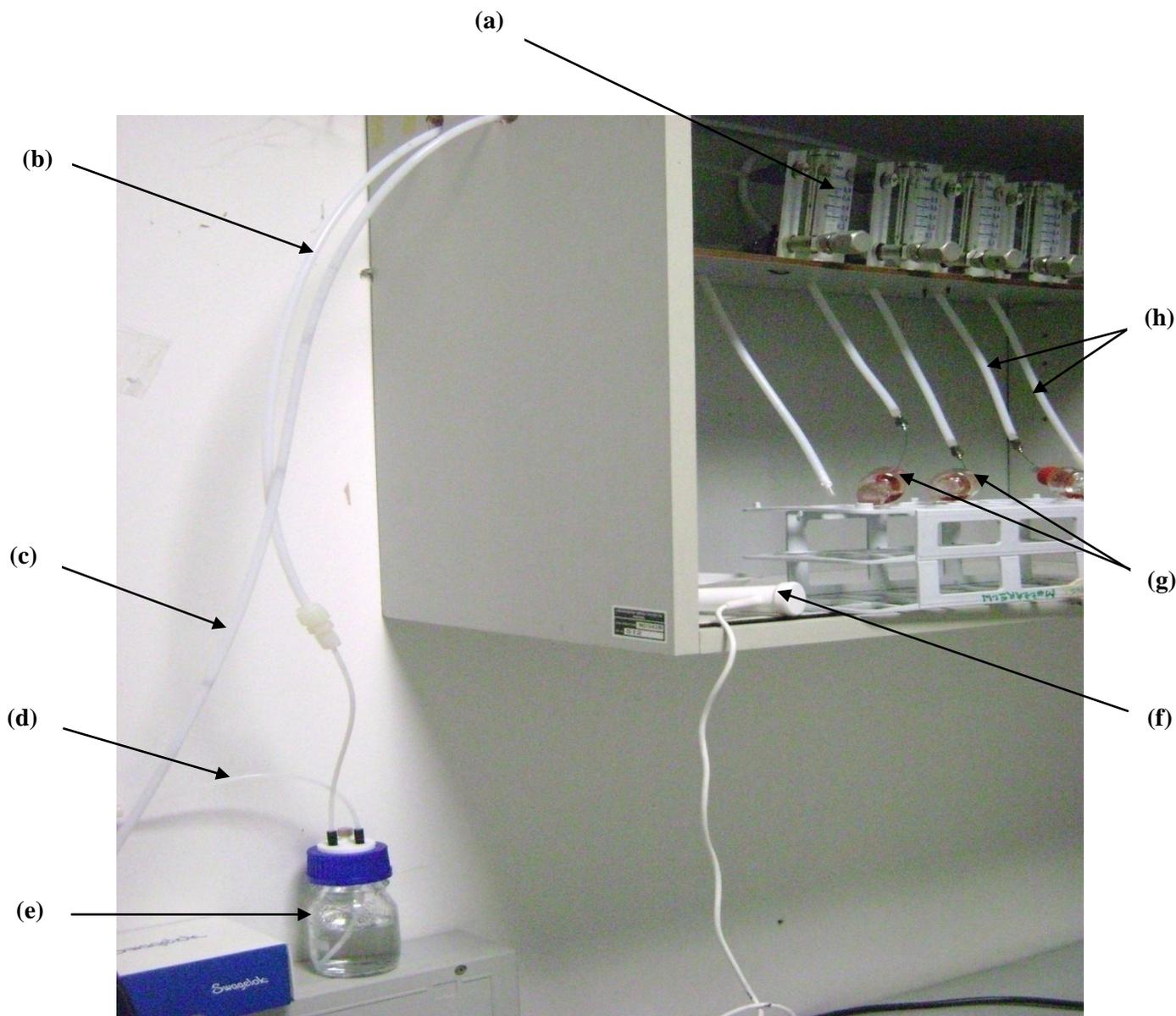
**Figure 3.3a: Set up for the deoxygenation of haemoglobin**
