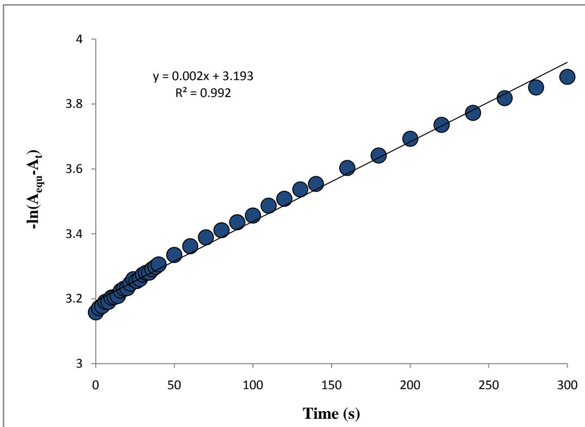
**Figure 4.24:** Semi-logarithmic plot of the time course for the reaction 5,5'-dithiobis(2-nitrobenzoate) with **stripped human deoxyhaemoglobin A** sulphhydryl groups in borate buffer pH 8.00;  $[DTNB] = 100 \mu\text{mol dm}^{-3}$ ;  $k_{\text{obs}} = (2.45 \pm 0.04) \times 10^{-3} \text{ s}^{-1}$ . The plot was linear for 1.1 half lives. Data from Figure 4.21.
