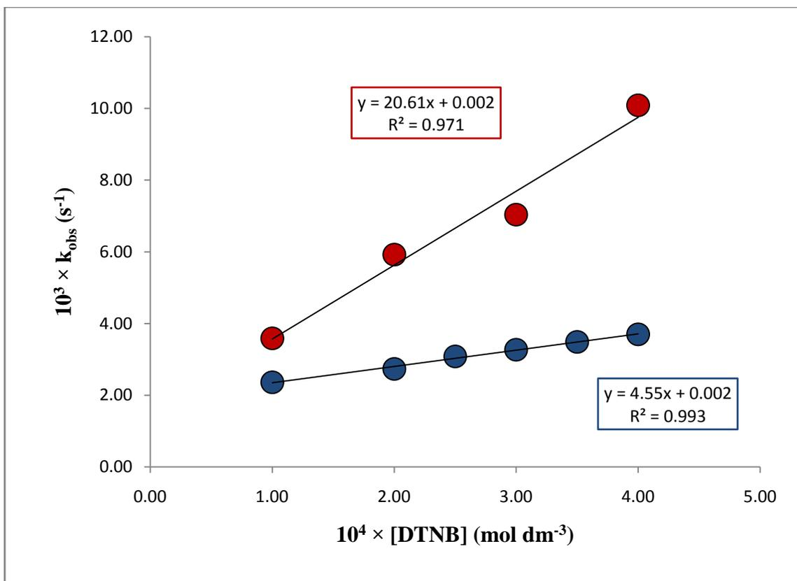
**Figure 4.28:** A comparison of the dependence of the pseudo-first order rate constant,  $k_{\text{obs}}$ , on the DTNB concentration for the reaction of DTNB with stripped human oxyhaemoglobin A (blue symbols) and deoxyhaemoglobin A (red symbols) at 25°C. Conditions: borate buffer pH 8.00; (ionic strength 50 mmol dm<sup>-3</sup>; added salt, NaCl); haemoglobin concentration, 10 μmol (haem) dm<sup>-3</sup> (5 μmol dm<sup>-3</sup> in reactive sulphydryl groups).
