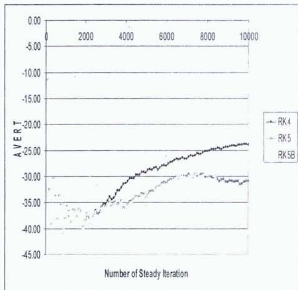
Figure 1: Variation of AVERT with number of steady iteration in hyper-chaos of Rösler using fourth order, fifth order and Butcher's modified fifth order Runge-Kutta methods and NRK1
